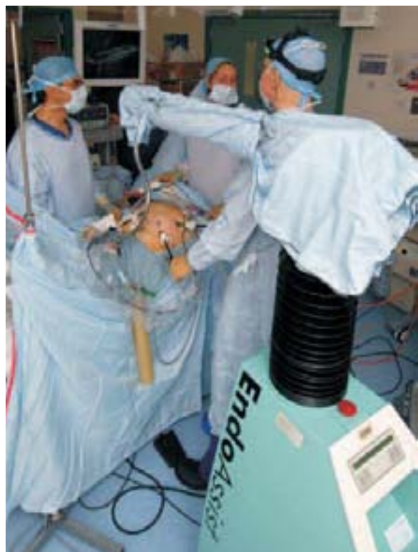
The EndoAssist robotic laparoscopic holder in use in a laparoscopic anterior resection of the rectum
